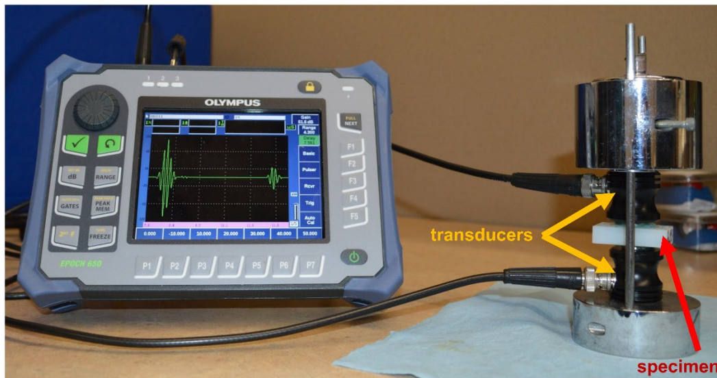
Fig. 5 Experimental setup showing an example of a measurement on a specimen from one of the panels. Measurement is in through-thickness mode (defined in Section 3.2.5) showing both the transmitting and receiving transducers. The transducers and specimen are held in place with a custom clamping device. Transducers are connected to the digital flaw detector used for generating and measuring waveforms. The waveform shown on the flaw detector is one of the best examples, showing clearly the first and second reflected pulses.
