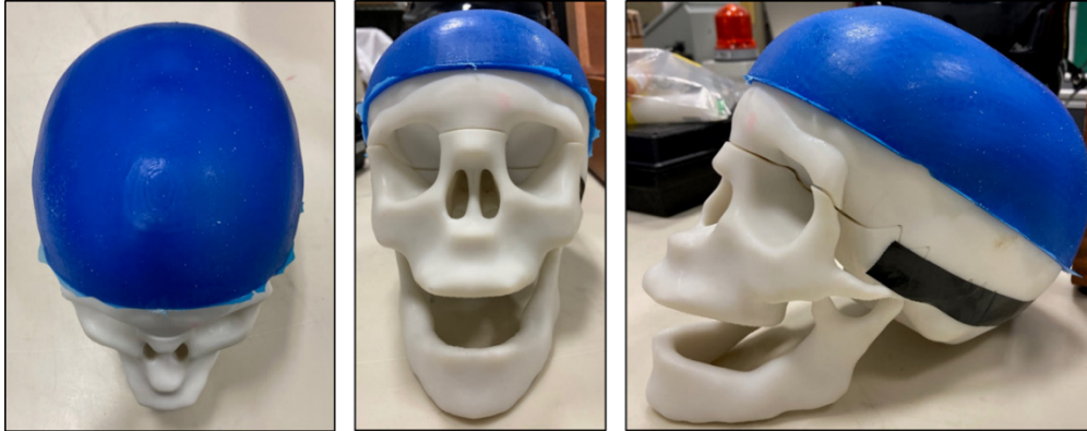
Fig. 5 Top, front, and isometric views of the skull cap placed on a surrogate skull
