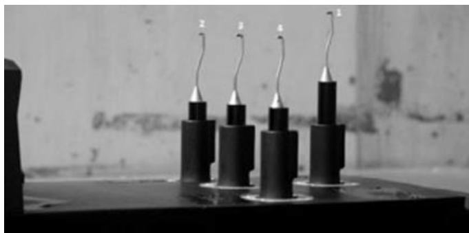
(b) probes used to measure airwake velocities
