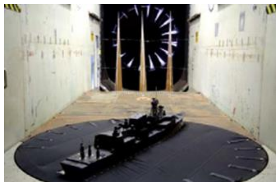
(a) wind tunnel setup
