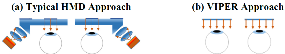
Figure 52: Simplified Diagram of (a) A Typical HMD Approach Using an Optical Relay System Versus (b) the Direct-view near-eye VIPER Approach
