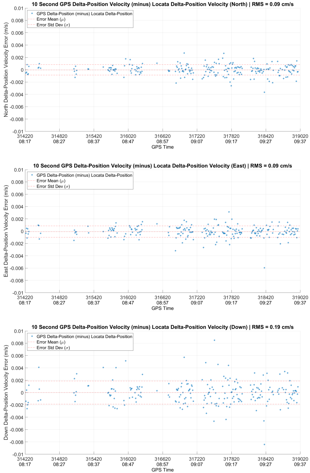
Figure 24: Comparison of 10 second averaged GPS delta-position velocity measurements and 10 second averaged Locata delta-position velocity measurements. Note that the vertical scale of these plots are \frac{1}{5} the scale of those in Fig. 23
