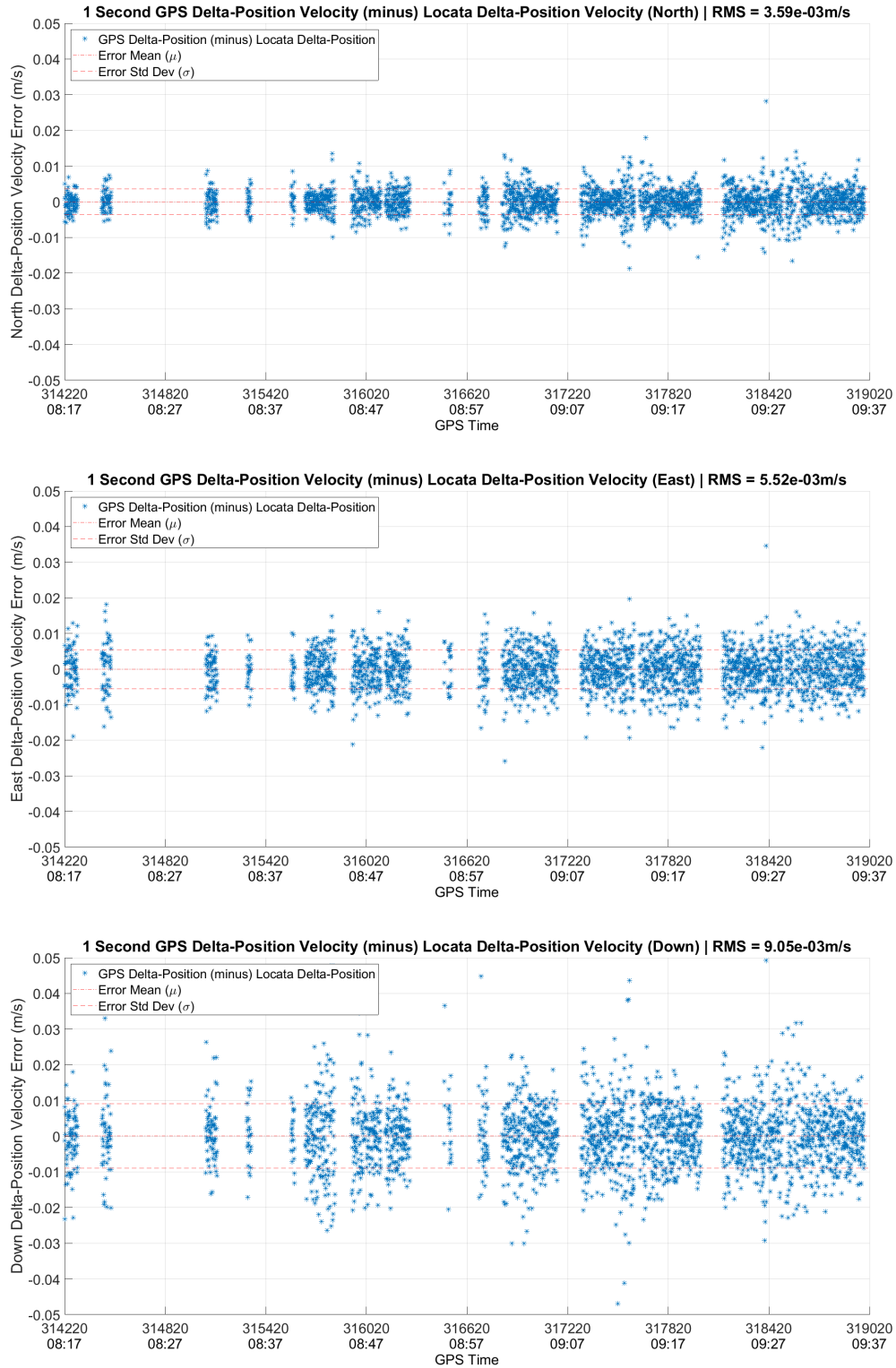
Figure 23: Comparison of 1 second averaged GPS delta-position velocity measurements and 1 second averaged Locata delta-position velocity measurements. Note that the GPS measurements are subtracted from the Locata measurements, and areas covered by red lines are periods of unavailability from either GPS or Locata.
