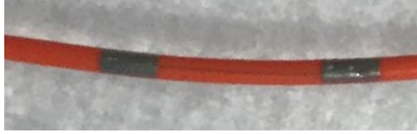
Figure 11. Contact pads with a single trace connecting them, printed on wire plastic casing.
