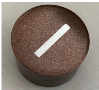
Figure 4. Cross-section of sample SN 36 potted in resin and polished.
