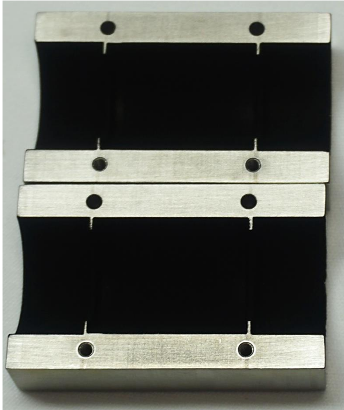
Figure 27. Stray light bore painted by NanoLab with Singularity Black LT Aero.
