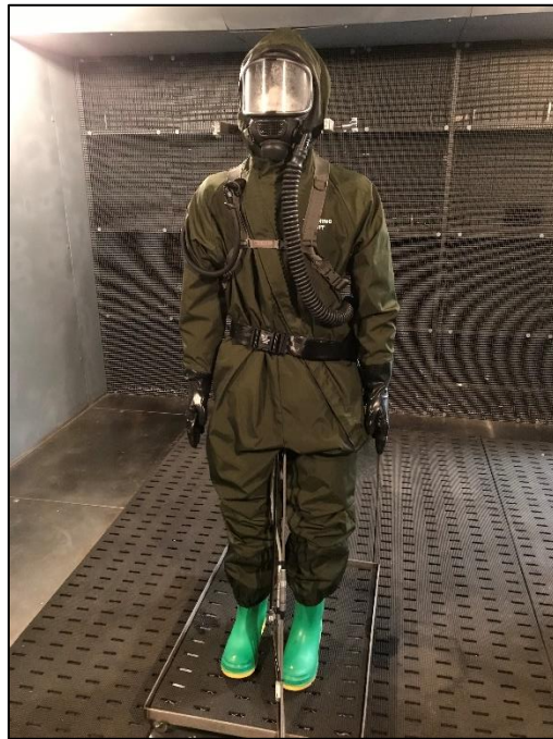
Figure 4. Thermal manikin wearing the Blauer XRT HAZMAT suit.
