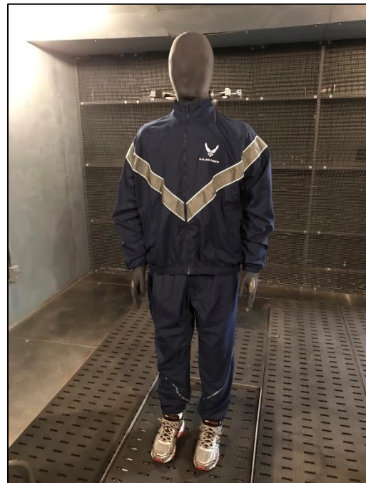
Figure 2. Thermal manikin wearing the Air Force summer and winter physical fitness uniforms
