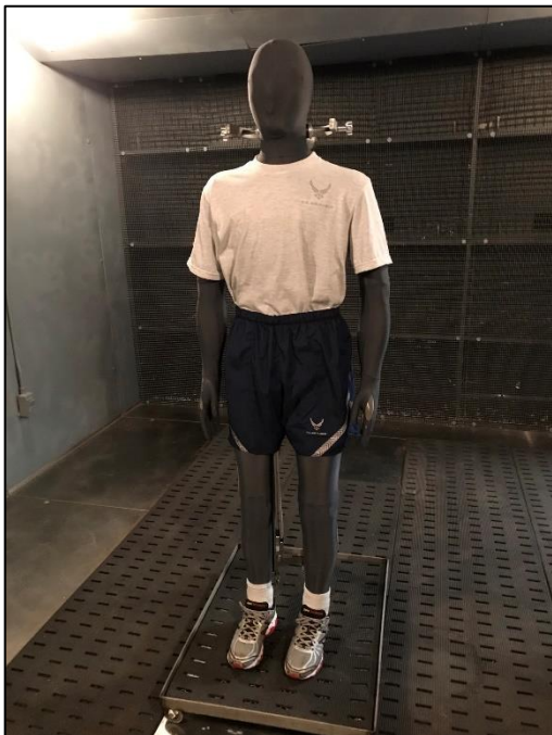
Figure 2. Thermal manikin wearing the Air Force summer and winter physical fitness uniforms
