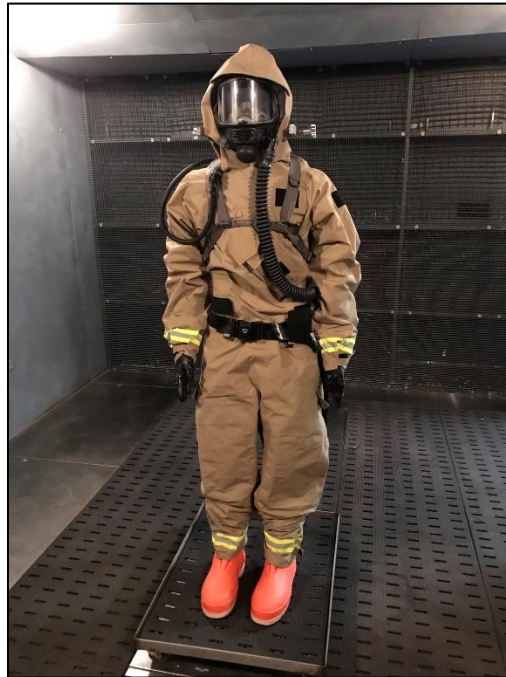
Figure 5. Thermal manikin wearing the Lion MT-94 HAZMAT suit.
