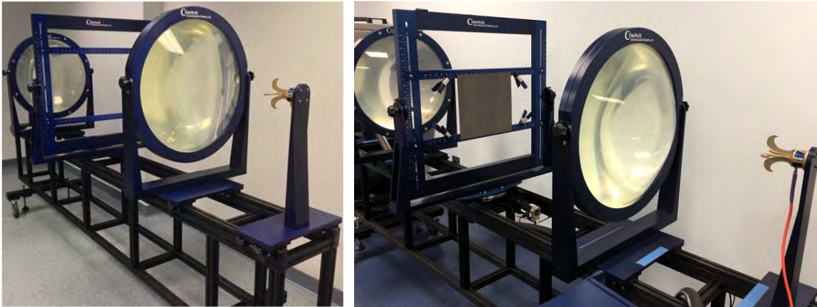
Figure 64. Typical focused beam system (FBS) configuration showing lenses, feed antennas, and sample mounting structure (left). Same system showing material coupon mounted within support frame (right). Used by permission. Photo courtesy of the Compass Technology
