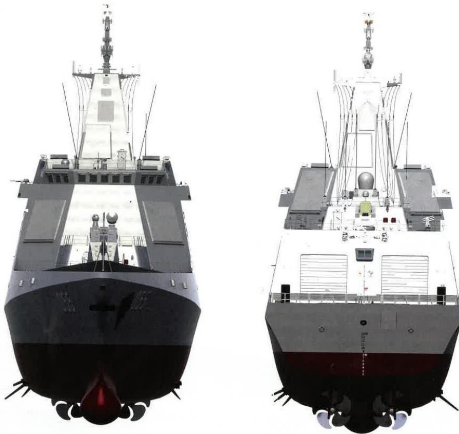
Image 10. Bow and stern views of the Type 055 reveal the large S-band planar arrays. The twin hangar doors also may be indicative of the PLAN’s new appreciation for the importance of shipborne helicopters for surface combatant operations. Source: Modern Ships 2017-5.
