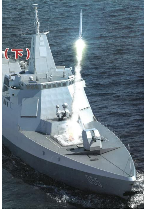
Image 7. A graphic image portrays the launch of a YJ-18 ASCM, a lethal missile based on the Russian SSN-27. The cruiser boasts a large magazine of 112 VLS cells. In addition to strong air and missile defense armament, therefore, the vessel is also a potent strike platform. Source: Modern Ships 2017-05.
