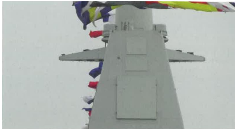
Image 4. The integrated mast of the Type 055 cruiser increases stealth and also incorporate an X-band radar. In combination with S-band planar arrays, the dual band radar sensor could be on par with the most advanced U.S. shipboard tracking systems. Source: Modern Ships , 2017-7.
