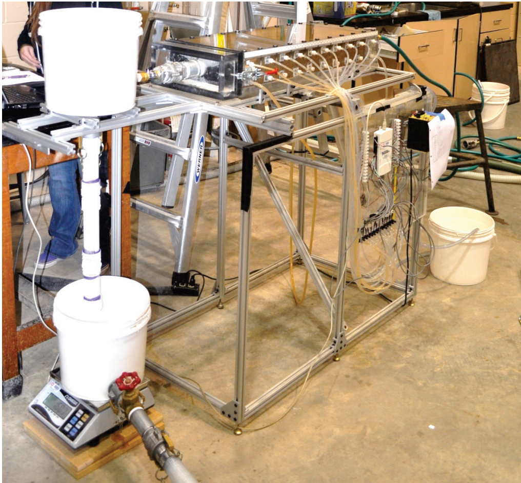
Figure 8. Complete setup of small flume with weighing scale.
