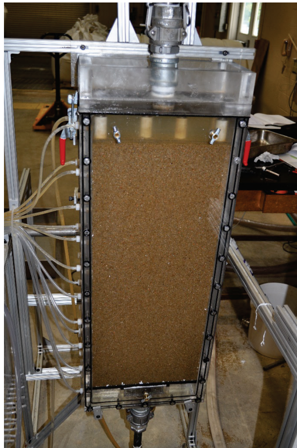
Figure 4. Small flume in vertical position after finishing the sample preparation.
