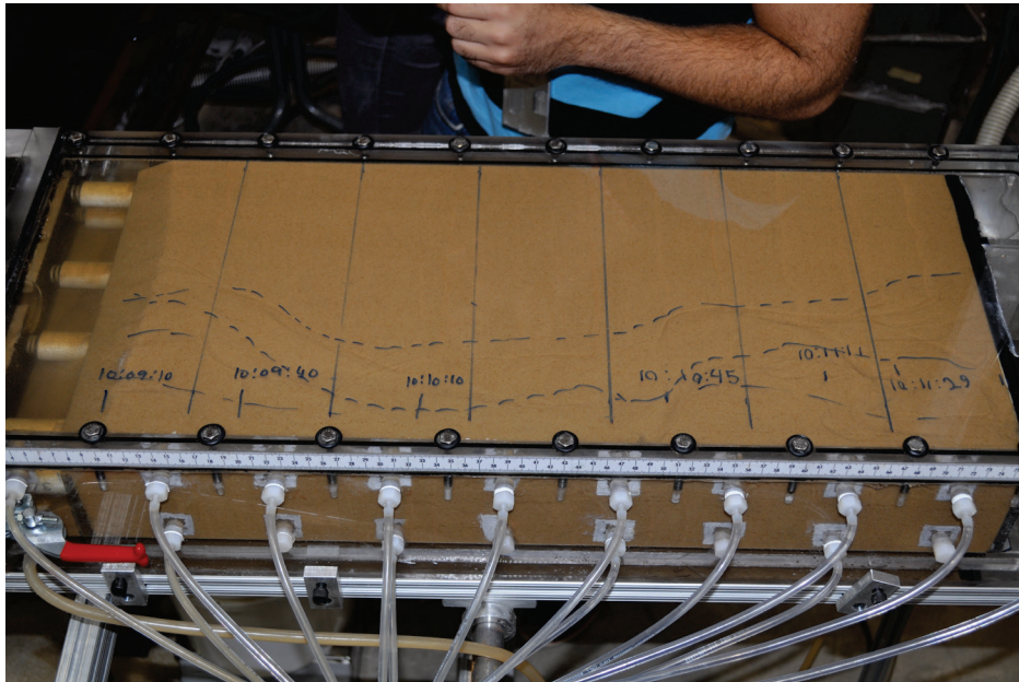
Figure 20. Final pipe path with pipe positions marked for Test 40-70-4.
