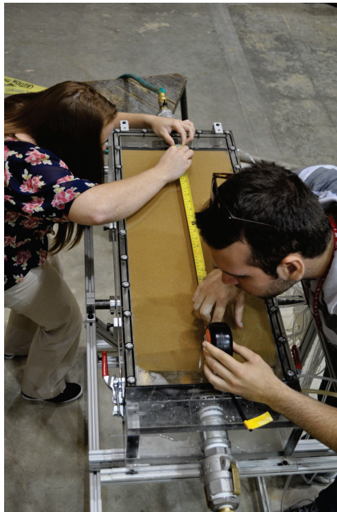
Figure 17. Measuring the shortest sample length (or seepage length) from the top of the sample with small flume in horizontal position.
