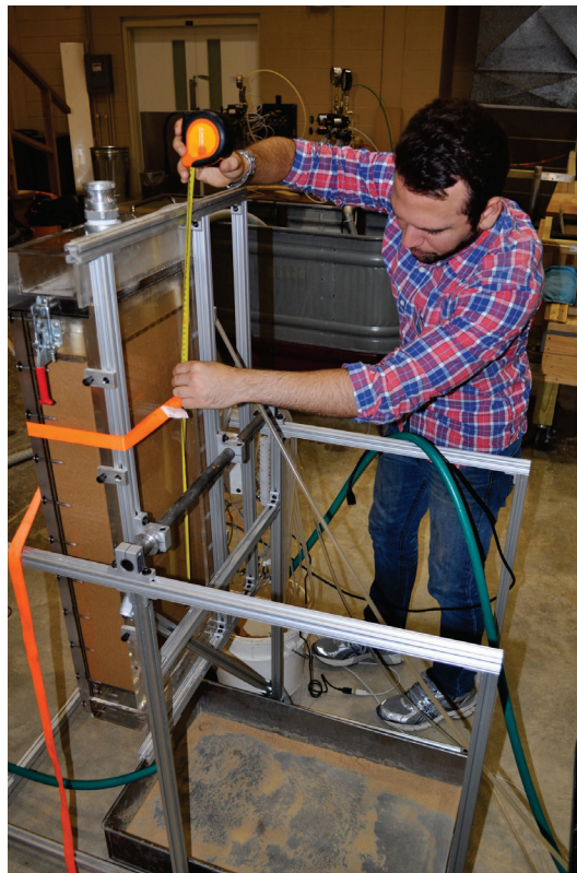
Figure 16. Measuring height of sample for the determination of volume.
