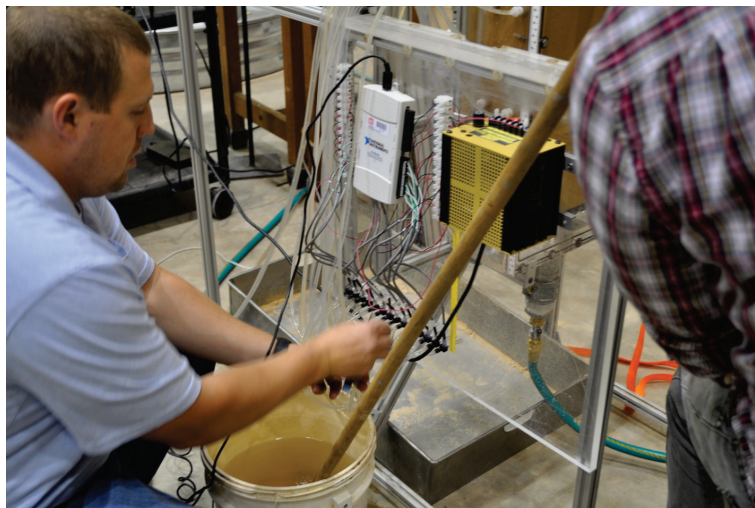
Figure 13. Draining tubes connected to the transducers for saturation.
