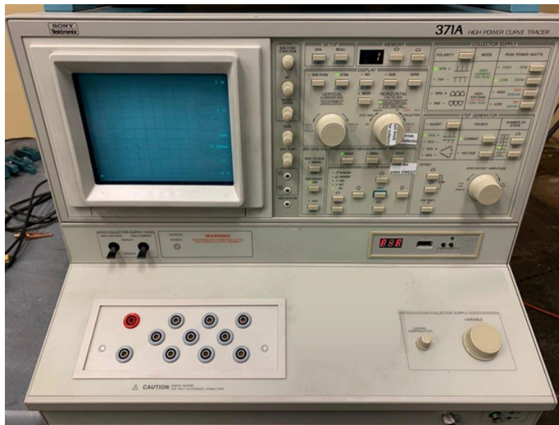
Fig. 1 Tektronix 371A with GoTek floppy drive emulator installed
