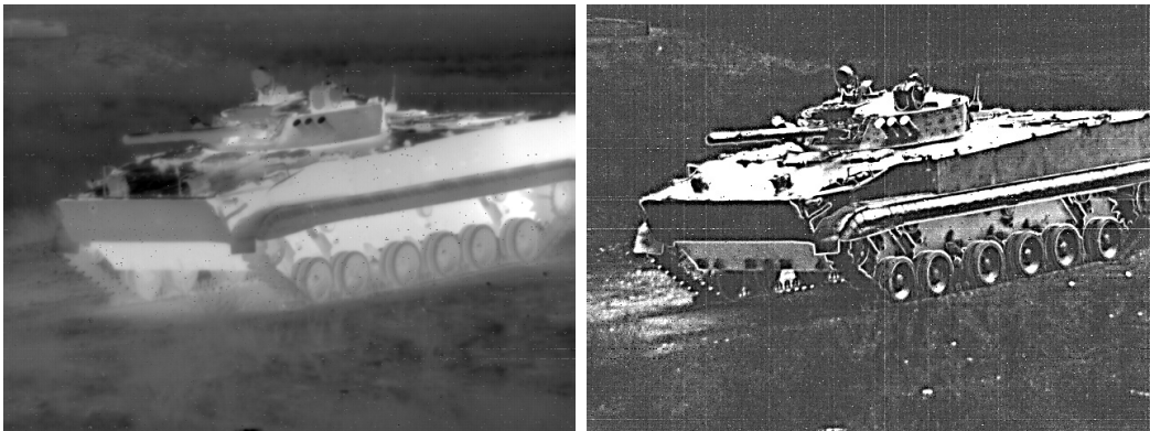
Fig. 2 LWIR thermal (left) and the resultant polarimetric DoLP image (right) comparison of a Russian 1970s vintage T-72 tank
