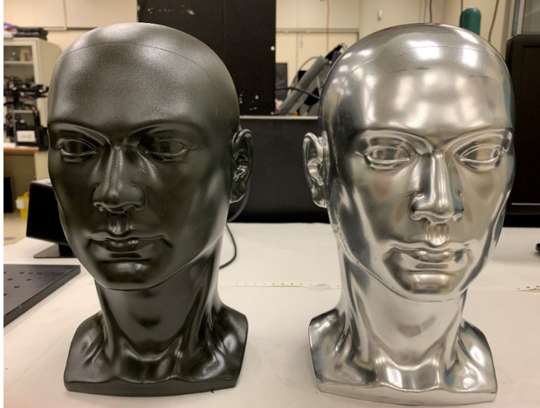
Fig. 6 Image of coated diffuse carbon-black manikin head (left) and coated mirror pigment manikin head (right) used as “emissive” and “reflective” targets, respectively
