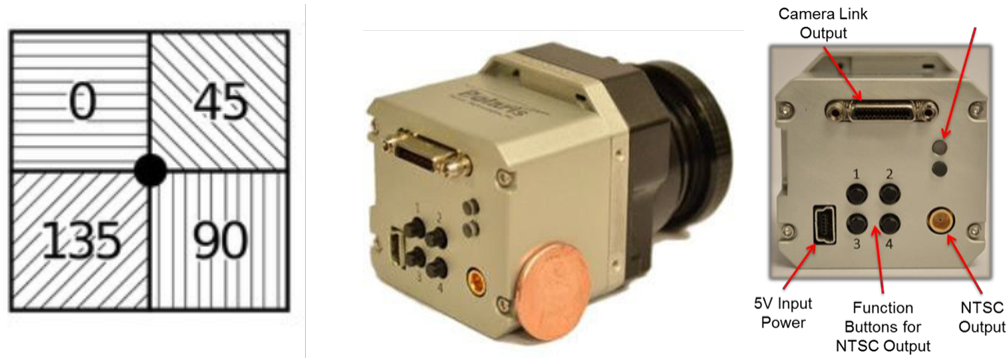
Fig. 2 Schematic of the micro-grid polarizer orientation geometry (left) and a photograph of the LWIR microbolometer-based polarimetric sensor (right) used in this study
