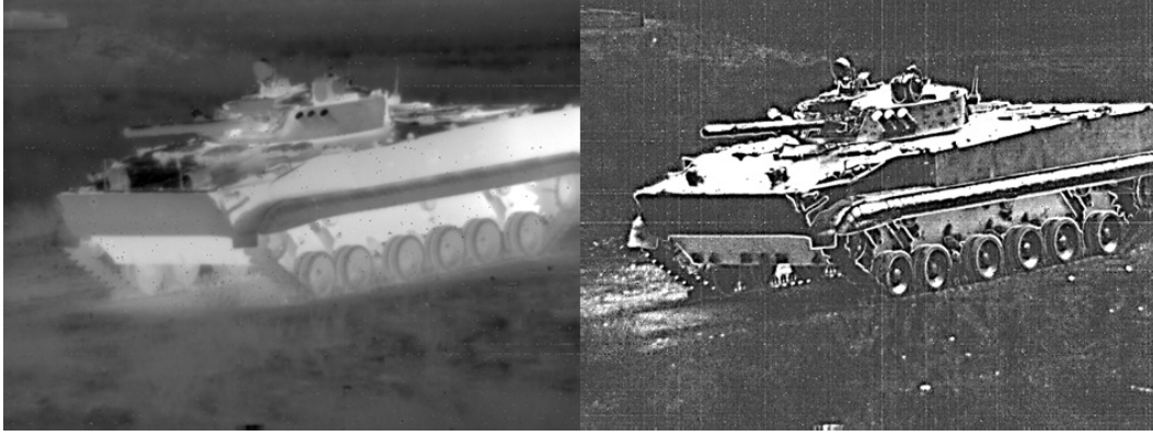
Fig. 1 LWIR thermal (left) and the resultant polarimetric degree-of-linear-polarization (DoLP) image (right) comparison of a Russian 1970s vintage T-72 tank
