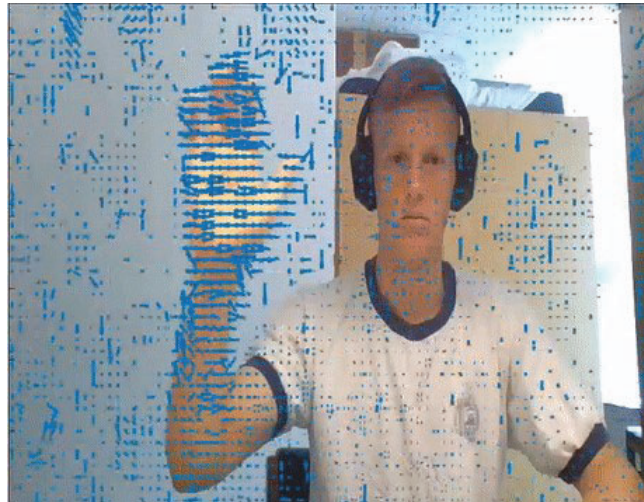
Figure 20: H.264 motion vectors extracted from an example recorded video of a moving hand. The direction and magnitude of travel of the macroblocks are represented by blue arrows.
