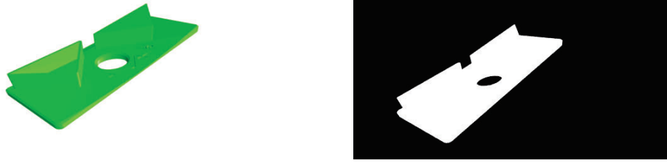
Figure 32: Left: Simulated image render of an AM product on the TAZ6 printbed. Right: The associated contour binary for the simulated image.
