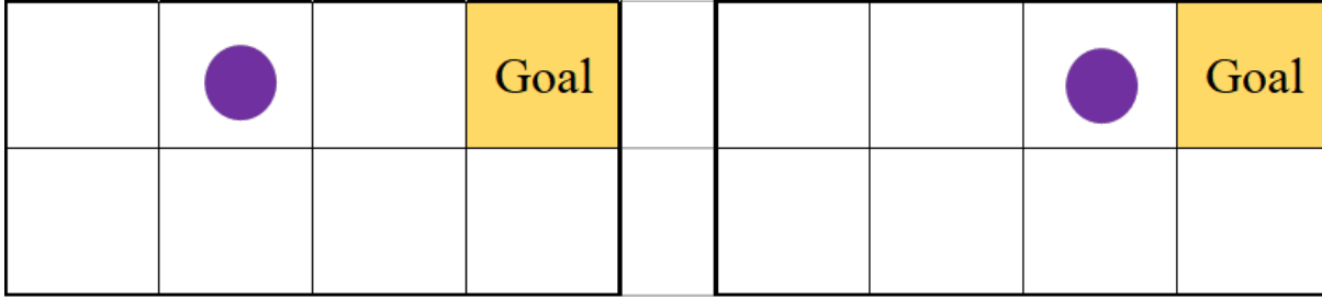
Figure 5.1: These 8 squares represent the environment in this simple example. The purple circle is the agent. The picture on the left represents State 1 and the picture on the right represents State 2. If the agent is in State 1, it can take the action of 'Move Right' and will reach State 2. The goal state or end state is when the agent is on the yellow square labelled Goal.
