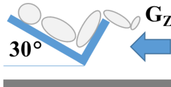
Figure 3. Seating orientation for experimental and computational tests conducted by Paskoff et al. (2004).
