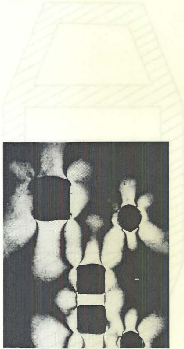
GLASS JOINT WITH CENTRAL HOLE PREPARED BY FUSION
