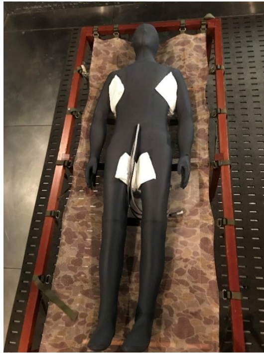
Figure 3. Thermal manikin with Polar ice packs only
