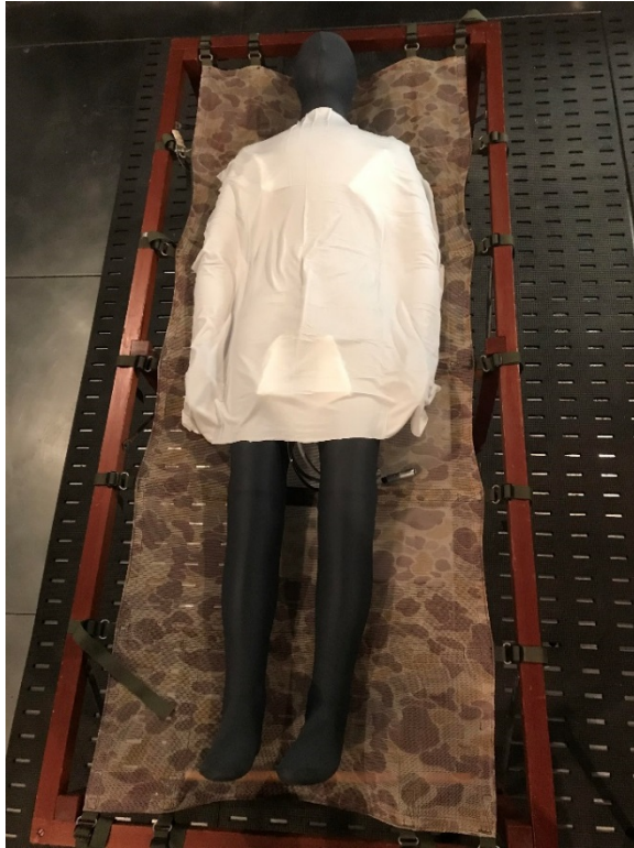
Figure 2. Thermal manikin with Polar ice sheet and ice packs
