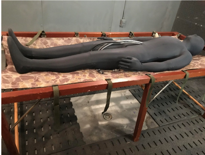
Figure 1. Thermal manikin without supplemental cooling
