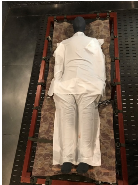
Figure 4. Thermal manikin laying on the cot with two Polar ice sheets and four Polar ice packs.
