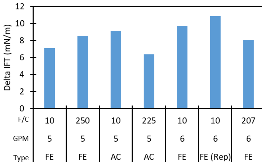
Figure 12. \Delta IFT of Fuel Due to Clay Treating for Diatomaceous Earth (DE), FE, AC; Flow Rates; and F/C Ratios
