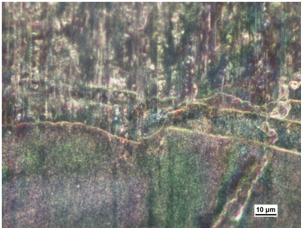
Figure 34. Dark field image of Al-S-MgG coating-substrate interface
