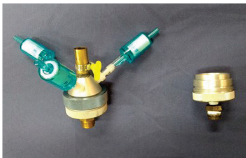
Figure 6. The 47 mm open-face filter holder (right) and closed-face filter holder (left). Three HEPA filters are attached to the closed-face filter holder to provide clean air to the system.
