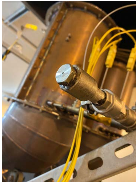
Figure 30. 1.5875 mm (1/16") Exit Nozzle Diameter Installed.
