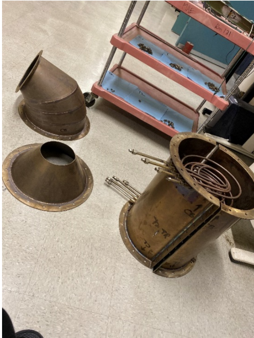
Figure 18. Modified Heat Exchanger Disassembly
