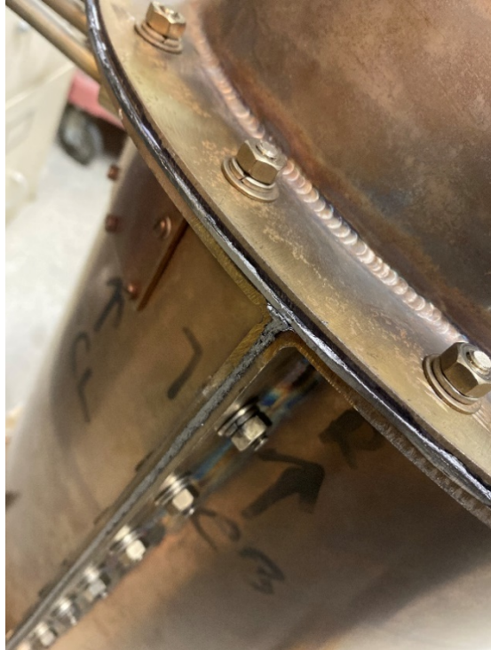
Figure 19. Close-Up View of Heat Exchanger with Installed Gaskets
