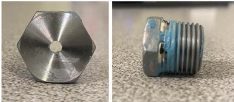
Figure 29. 1.5875 mm (1/16") Exit Nozzle Diameter
