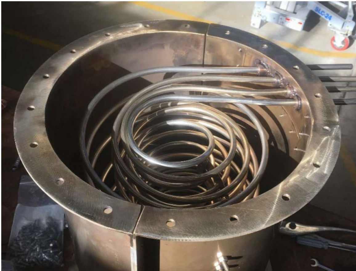
Figure 16. Kaim's Modified Heat Exchanger. Source: [6]
