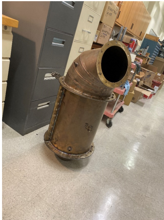
Figure 20. Heat Exchanger Full Reassembly with Installed Gaskets
