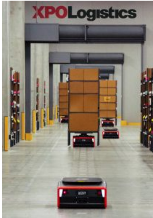
Figure 9. Collaborative Robots (Cobots) Carrying Batches of Items in MSUs. Source: XPO Logistics (2019a).
