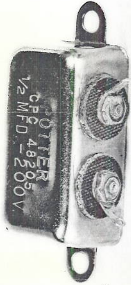
Potter capacitor under test, received from I.N.M., Chicago. Terminal seal satisfactory.
