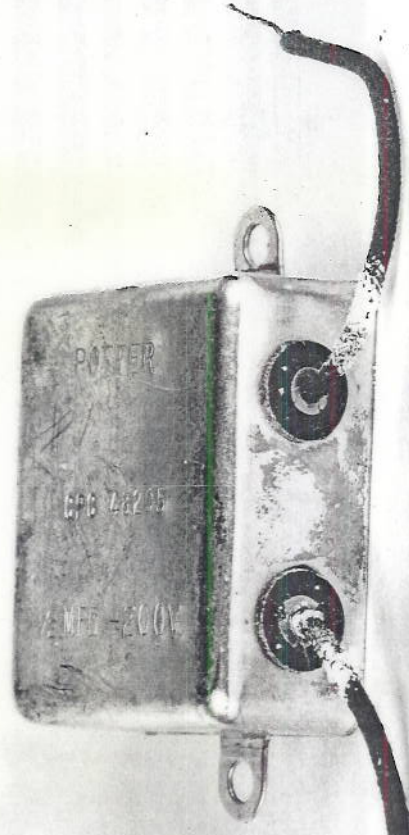
Potter capacitor submitted to N.R.L. by manufacturer. Terminal seal unsatisfactory.
