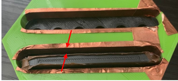
Figure 9. Gaps between copper tape and bar.
