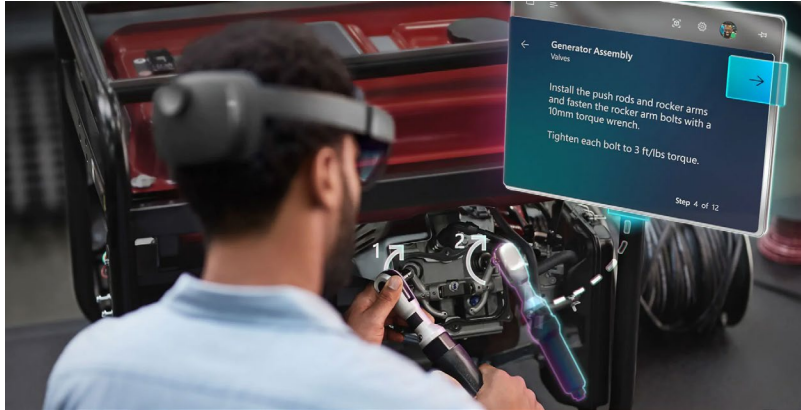
Figure 1. Maintenance Person Using the Microsoft HoloLens 2. Source: Microsoft (2020).
