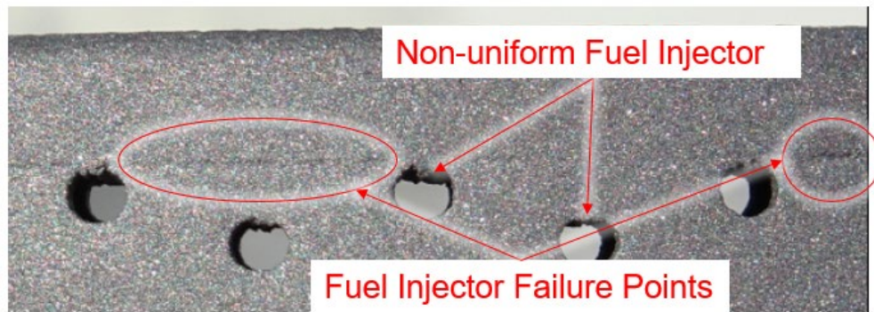
Figure 42. Fuel Injector Non-Uniformities and Failure Points. Source: [16].
