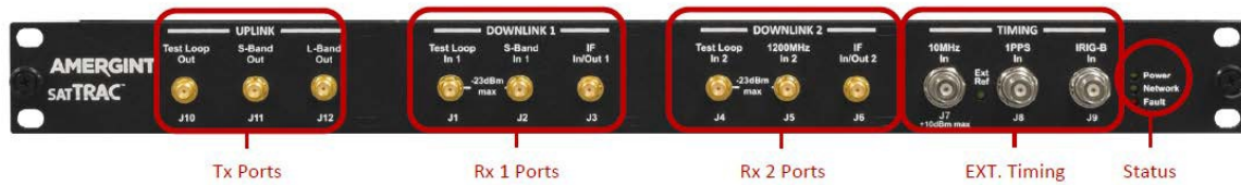
Figure 26. Depiction of satTRAC signal converter front plate. Source: [26].
