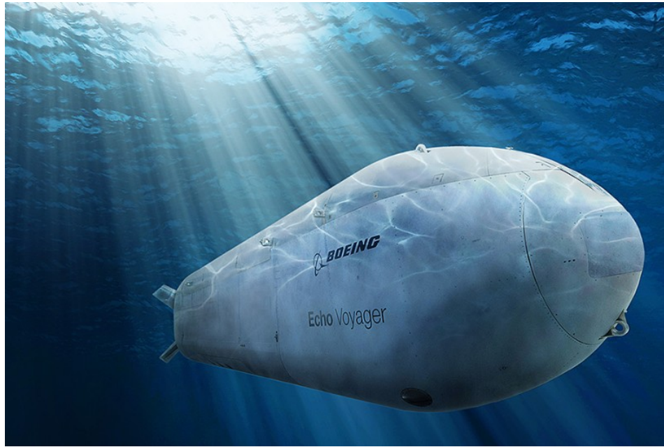
Boeing's Orca design is based on its previously developed Echo Voyager XLUUV, which can perform duties at sea for months at a time.
