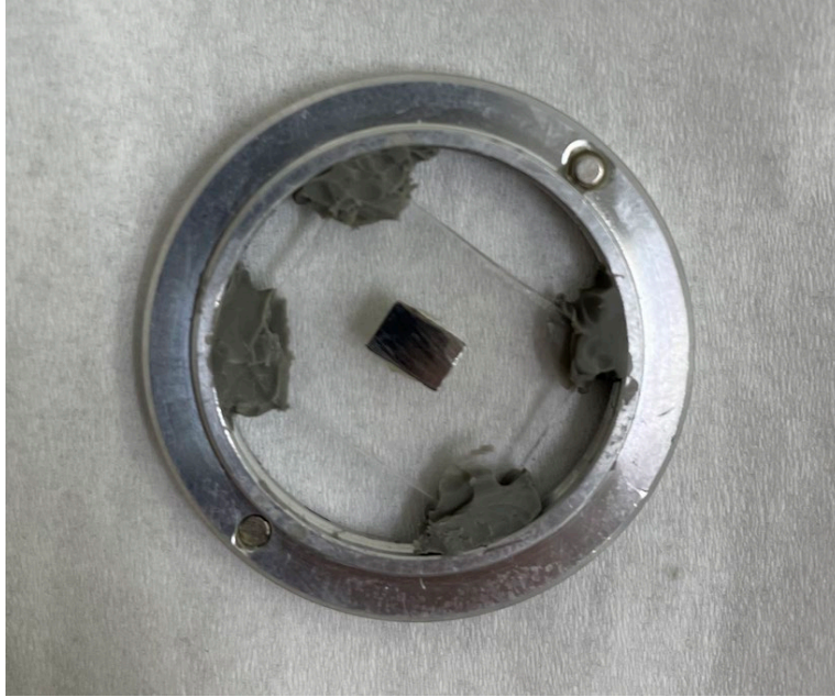
Figure 23. Coupon segment mounted for XRD analysis
