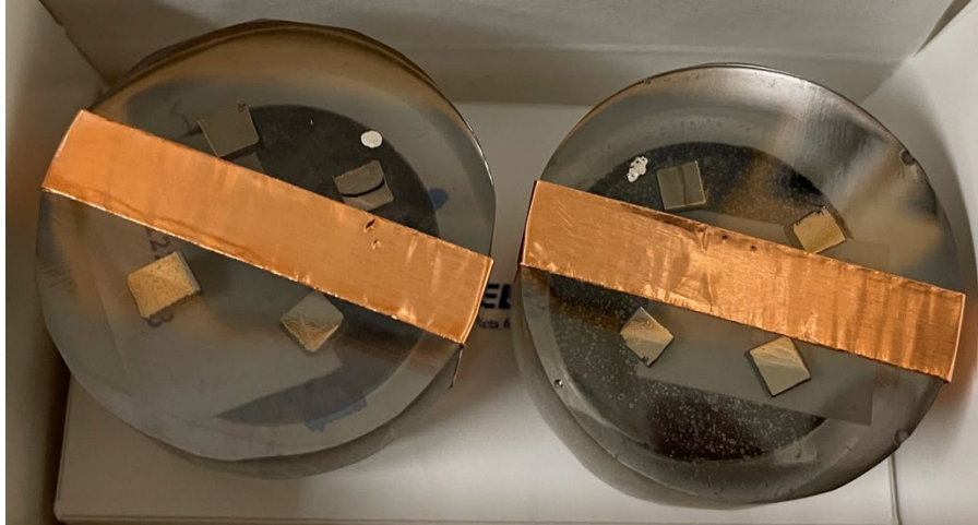
Figure 21. Mounted, polished, etched, and sputter coated samples prepared for SEM analysis
