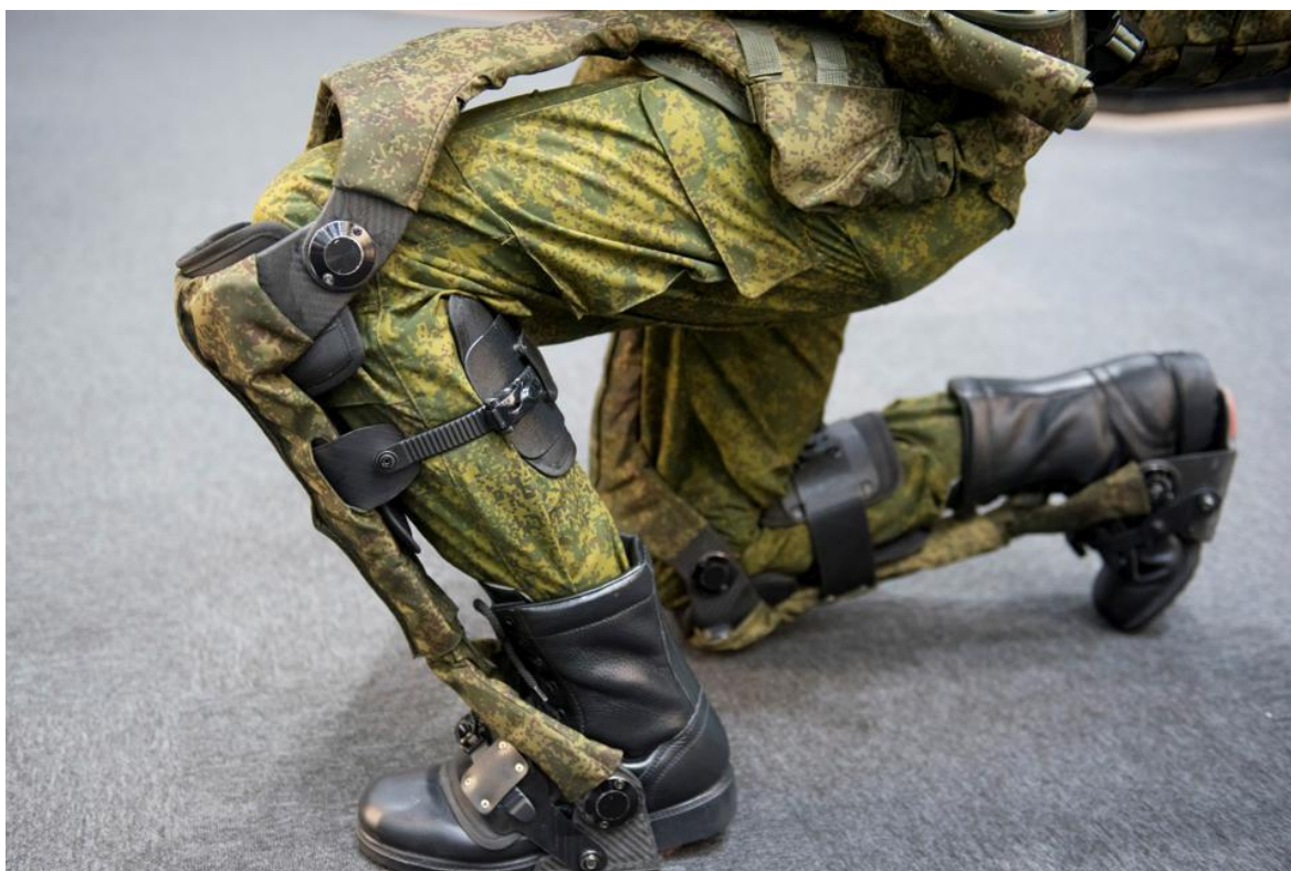
Figure 13. Example of ROSTEC's Ratnik Exoskeleton (passive)
