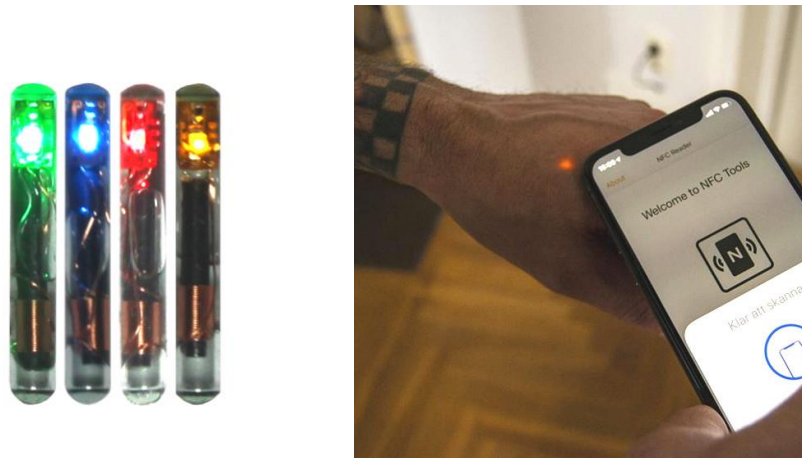
Figure 18. NFC implants with LED (left) and installed in a hand (right)
