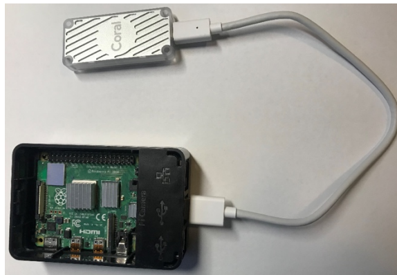
Figure 1. Raspberry Pi v4 with Coral TPU accelerator connected by USB 3.0.
