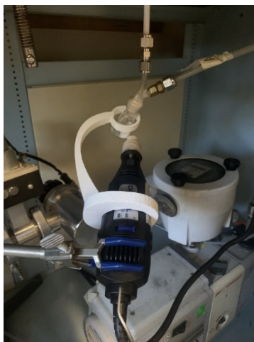
Figure 13. Final iteration for agitator setup utilizing a custom 3D-printed part
