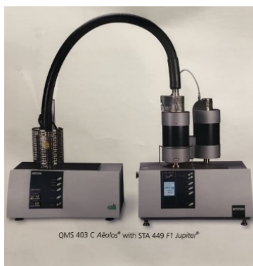
Figure 6. STA and QMS used for thermal analysis of zinc nitrate decomposition. Source: [16].
