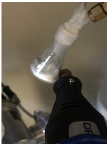
Figure 12. Second iteration of the vibration system. A rotary power tool with oscillating block positioned on the corner of the beaker containing precursor.
