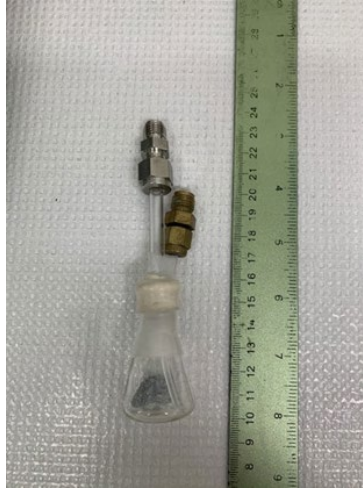
Figure 9. A beaker holding precursors with tubes for aerosol and carrier gases inside
