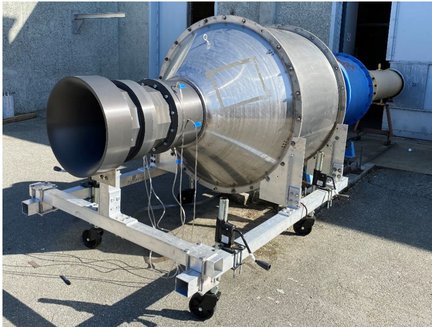
Figure 43. Manufactured support structure attached to the throttle casing and bell mouth
