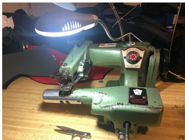
Figure 32. Blind stitch sewing machine for wetsuits
