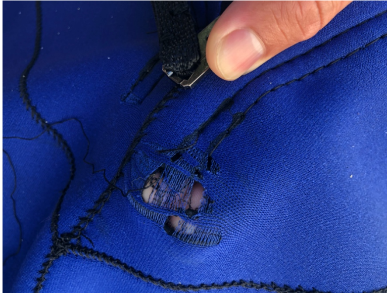
Figure 37. Hole in the back of the composite wetsuit
