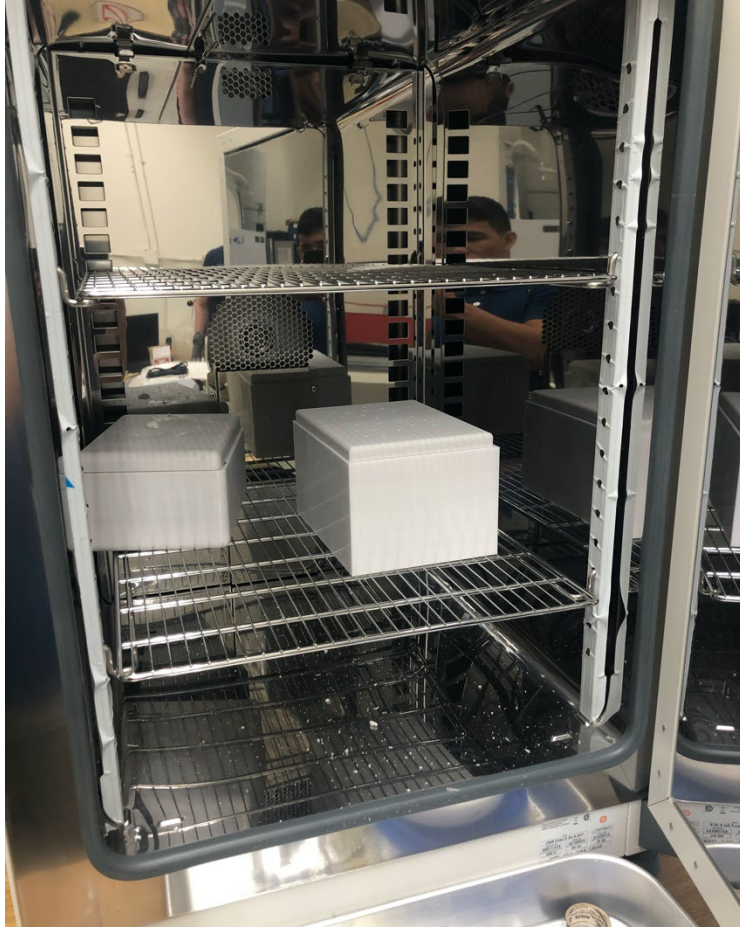
Figure 28. Molds with liquid composite being placed in the oven
