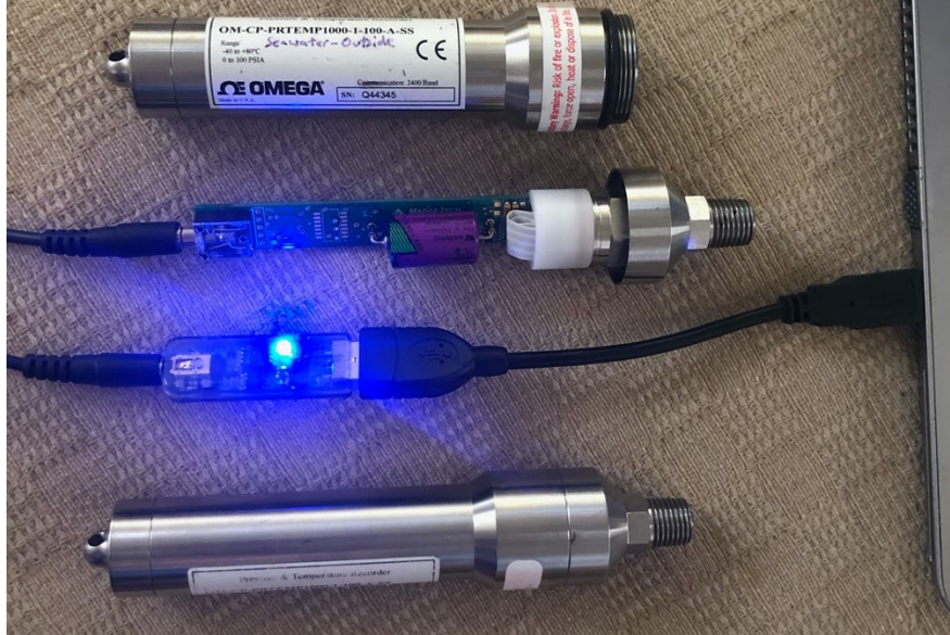
Figure 35. OM-CP-PRTEMP1000 pressure and temperature data loggers
