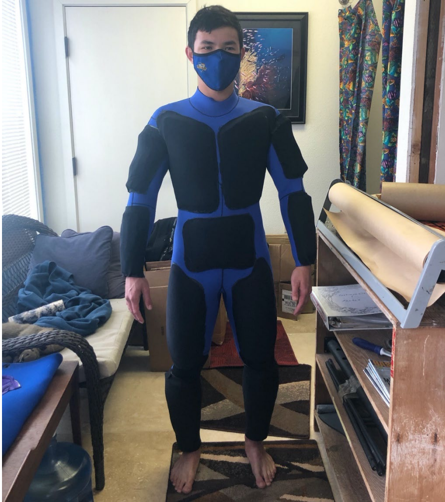
Figure 34. Finished composite wetsuit
