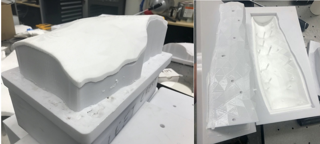
Figure 29. Left chest mold (left) and right shin panels (right) stuck to the top and bottom molds, respectively
