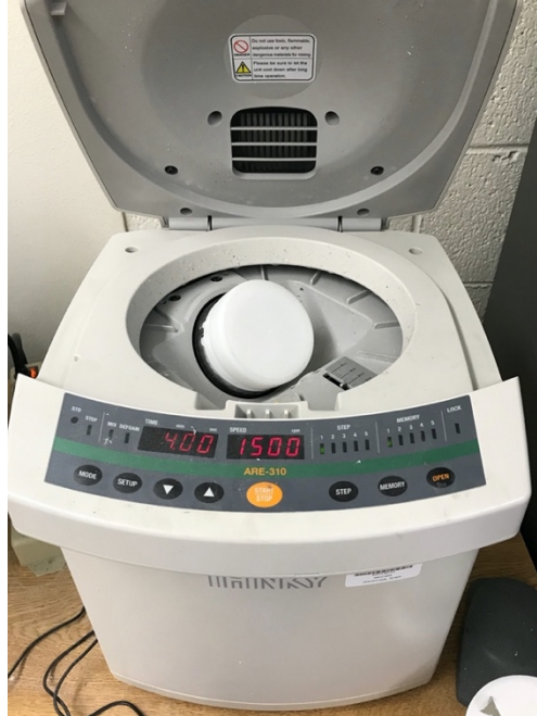
Figure 26. Rotary mixer ready to mix the casting material for four minutes at 1500 rpm
