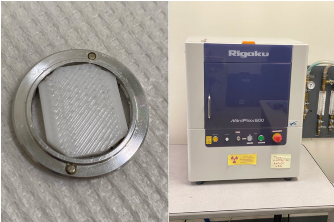
Figure 13. Example of PC sample mounted in tray for XRD analysis (left) and Rigaku Miniflex 600 XRD (right)
