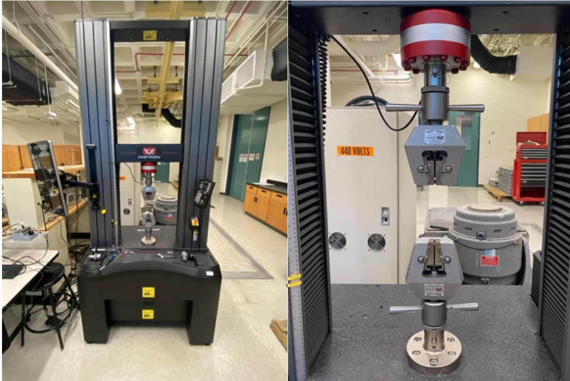
Figure 11. Instron: 5982 Universal Testing System (left) and Instron: 100kN Mechanical Wedge Action Grips (right)
