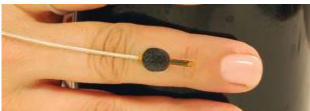
Figure 6 The Polhemus micro sensor is a 1.8 mm outer diameter magnetic sensor which is on a flexible cable. The device can be easily mounted to forceps with an adhesive or fixing pad.
