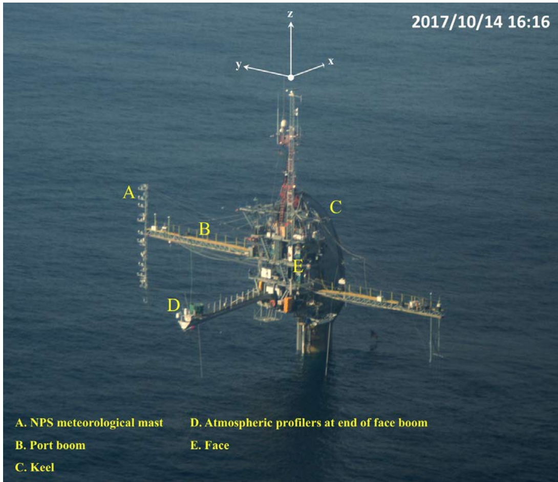
Figure 7. FLIP during the CASPER-West experiment with several features highlighted. Note that the heading of FLIP is the direction the keel points (x). The platform coordinate system is also given. Photo credit: D. Khelif, University of California at Irvine. Source: Ortiz-Suslow et al. (2019).
