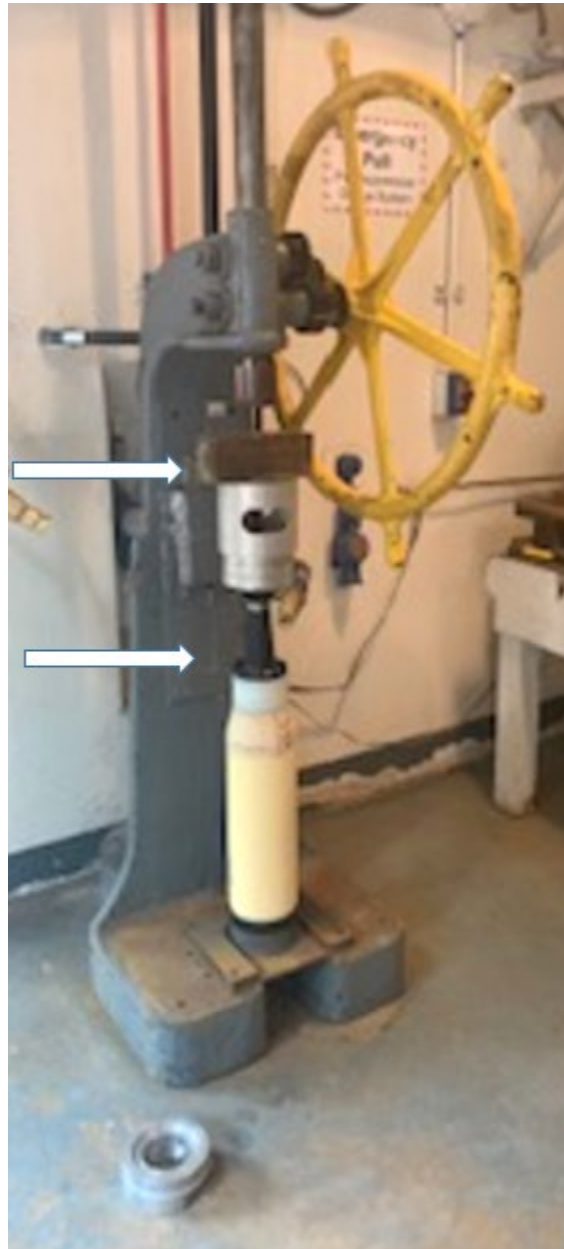
Fig. 9 Arbor press for seating projectile fully into cartridge case. Spacers indicated by top arrow, projectile by bottom arrow.
