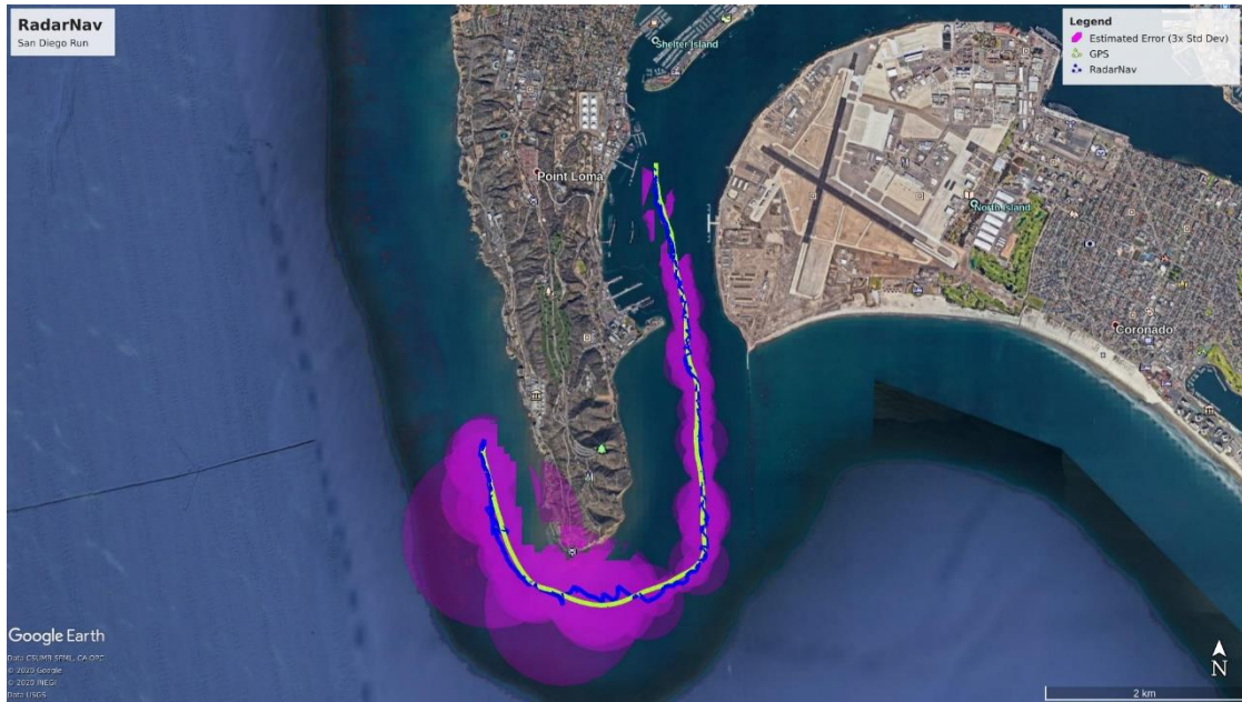
Figure 25. Map of RadarNav, GPS positions & estimated error for San Diego, CA.
