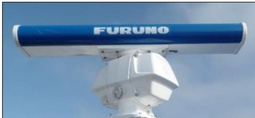
Figure 2. XN12AF radar antenna on RadarNav boat.
