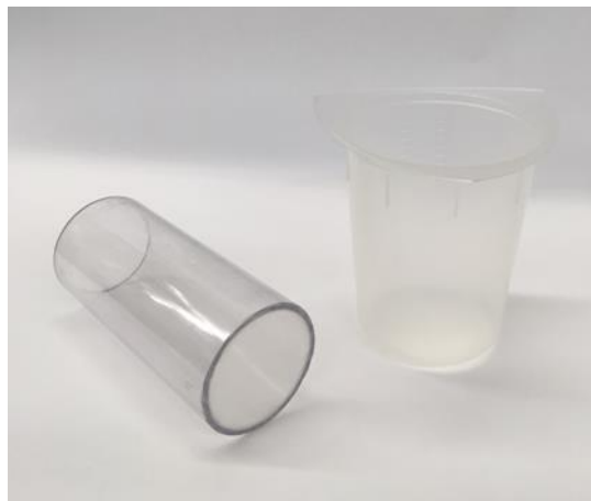
Figure 7-1. Nitex mesh screen tube and tri-corner beaker used for housing and transferring organisms during pulsed exposure toxicity testing.
