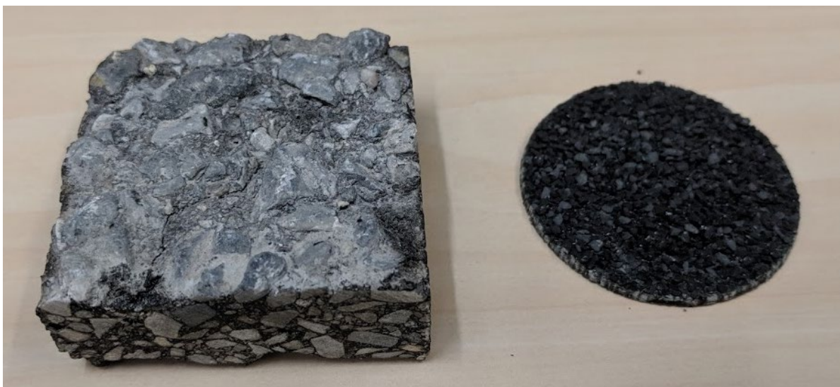
Figure 4. Thick asphalt sample from local roadway (left) and asphalt shingle coupon (right).
