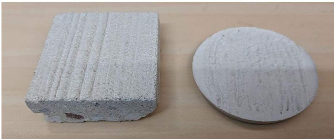
Figure 3. Thick concrete coupon (left) and 1/8 in. thick CSA quickset coupon (right).
