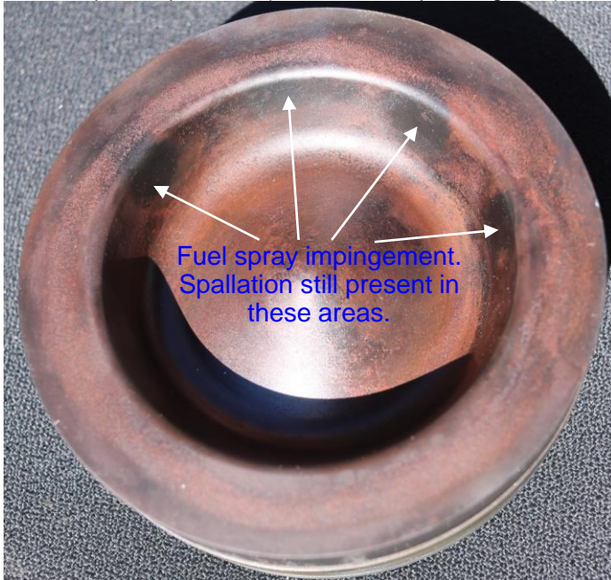
Build 34 piston, post-test (100 hrs total operating time)
