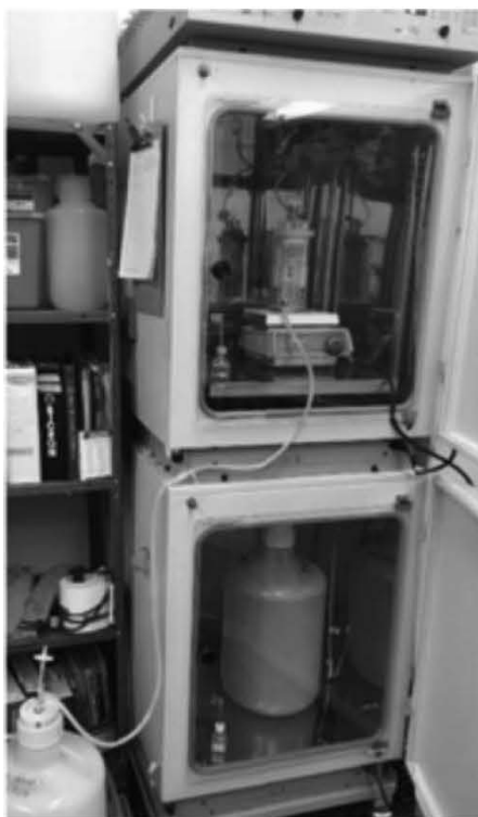
FIG. 5 Equilibrate Continuous Flow Growth Medium by Placing Carboy into an Incubator 2 to 3 Days Prior to Use
