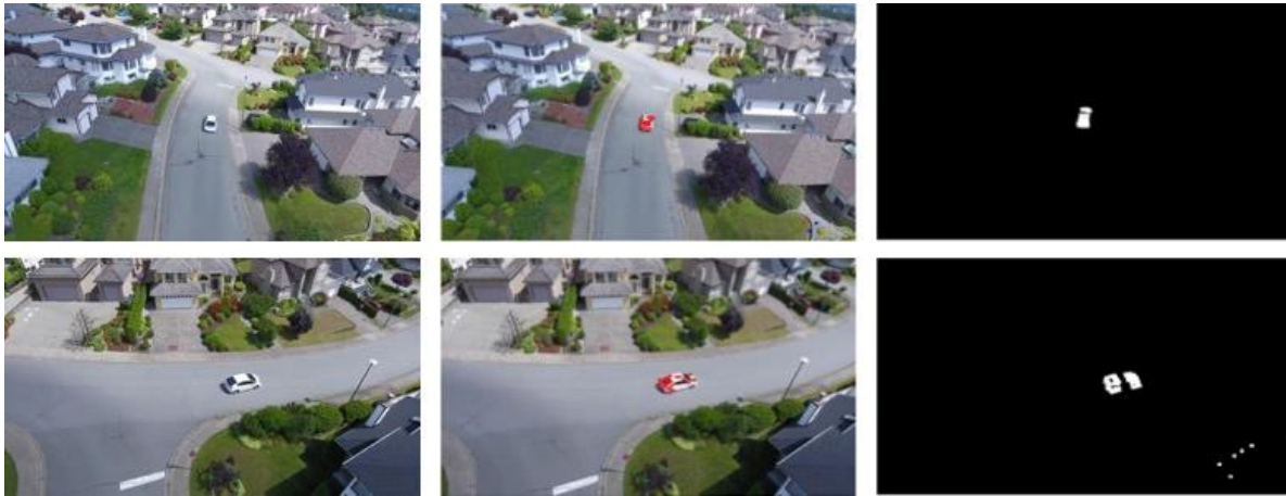
Figure 3: Illustration of DMD method for feature based and direct method for UAV video. Left: original input images from video sequence; Center: feature based DMD separation of background/foreground (red blobs indicates foreground features consistent across frame window, blue blobs are only for the current frame); Right: Foreground mask for the direct method using DMD.
