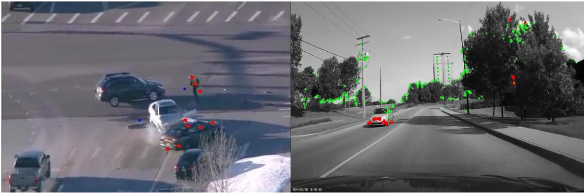
Figure 7: Examples of feature based background/foreground separation for UAV video (left) and dash camera video (right).
