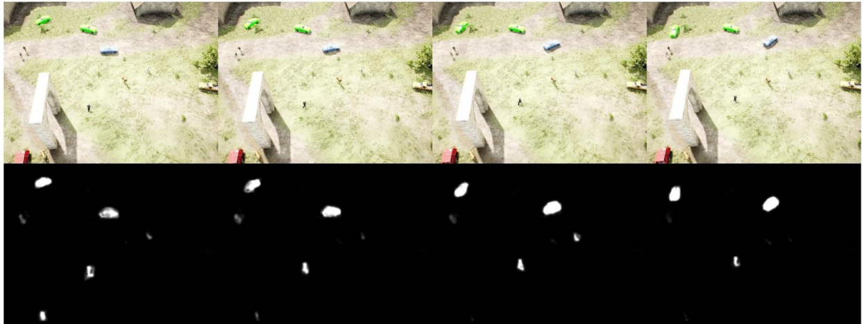
Figure 20: Background-foreground separation results on a synthetic video from a simulated camera on a UAV platform.
