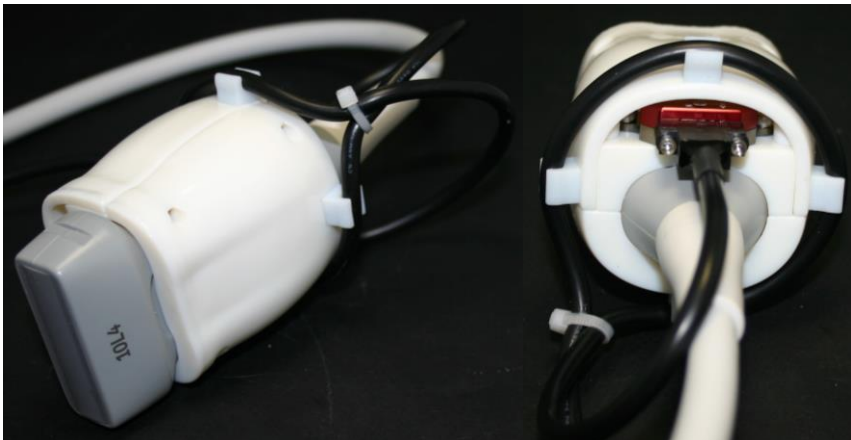
Figure 2: Mount for IMU on the 10L4 Sequoia ultrasound probe.
