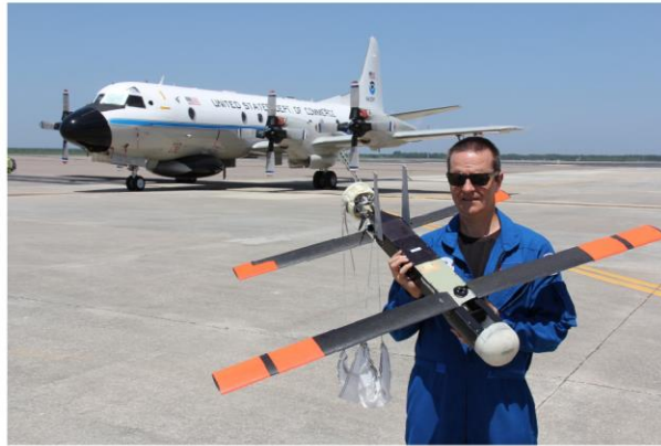
Figure 3. Coyote employed for hurricane research; launched from the P-3 in the background [18] (Figure courtesy of NOAA).
