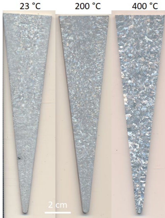
Fig. 3 The macro-etched structure for center slices of wedges produced at different Cu mold preheats
