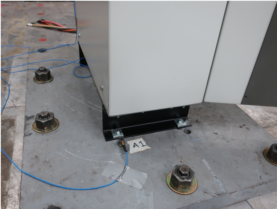
Figure B-2. Bottom left (south) side of the STS showing the A1x, A1y, and A1z accelerometers installed at the bottom left corner.
